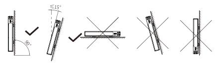
In order to ensure good heat dissipation and convenience in operation and maintenance, sufficient clearance shall be reserved while installing the battery. An example of such clearances are shown in the figure below. Please strictly follow the local battery installation guidelines, where applicable.
